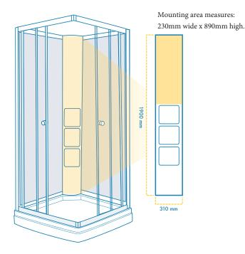
The Plain/Universal cabin is suitable for any type or wattage of electric shower or tap fitting as long as there is physically enough room to mount it on the corner column. The shower is supplied with a clamp on adjustable shower rail that can be fitted anywhere on the rear wall panels.
