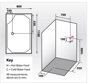
**Note.** The measurement shown on the floor of the diagram above is where the trap will be when the unit is in position. The plan features a right sided model, in a left sided unit the panel containing the mixer tap is located on the opposite side and the water connection points change accordingly.
