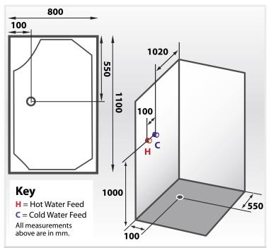
**Note.** The measurement shown on the floor of the diagram above is where the trap will be when the unit is in position. The plan features a right sided model, in a left sided unit the panel containing the mixer tap is located on the opposite side and the water connection points change accordingly.
