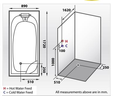
**Note.** The measurement shown on the floor of the diagram above is where the trap will be when the unit is in position. The plan features a right sided model, in a left sided unit the panel containing the mixer tap is located on the opposite side and the water connection points change accordingly.
