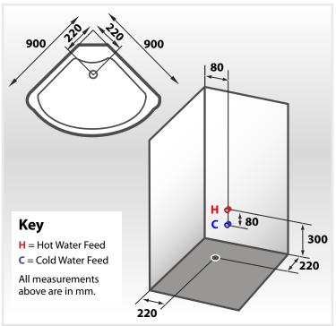
**Note.** The measurement shown on the floor of the diagram above is where the trap will be when the unit is in position.
